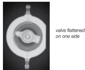
Fig. 19b: X-ray image adjustable DP-unit: setting 0 cmH 2 O
